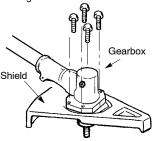
Insert and thread the 4 mounting screws through the holes of the gearbox and the metal shield. Tighten evenly and securely with the hex wrench provided.
